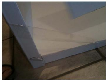
8. Lay box on its end, apply glue, lay in a 4 ft x 1 ft end section (trimmed if necessary to fit smoothly,) apply weights, let it set for a couple hours
