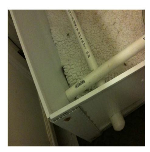
15. Cut edging to fit sides of box, press into place to cover sharp edges
